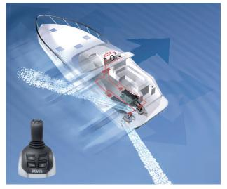
With the joystick the driver can now maneuver the boat, at low speed. The joystick is coupled to a sophisticated and specially developed software that individually commands the electronically controlled engines and underwater units of the system to steer, throttle and shift gears independently, making the boat move in any direction the driver wants – sideways, diagonally, forward, backward or rotate – with just one hand.
