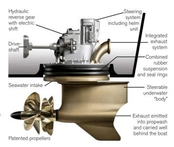
The Volvo Penta IPS has been developed and is manufactured as a complete system with everything included – engine, propulsion unit incl. gear box, propellers, exhaust and seawater system, steering, and controls.
